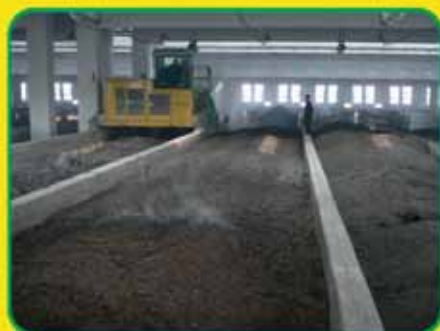
Tunnel-kompostipöorel (Lane Turner) Backhus LT 45 50 DC
